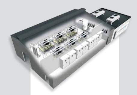
A 2MW installation: 2 lines of 3 HySTAT® 60 with a total production of 360 Nm³/h of high quality hydrogen. Each line has on large purification system, one closed loop cooling system, one feed water treatment system and is operated by one control panel to offer redundancy.
